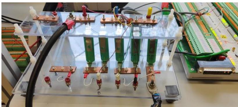
Figure 3: Battery pack made of 5 cells in series.
