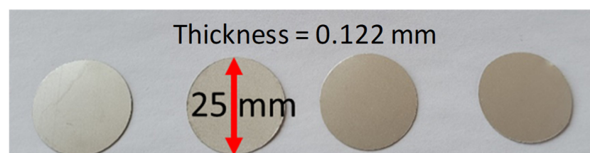
Figure 1. PVDF transducers cut into a disk shape.
