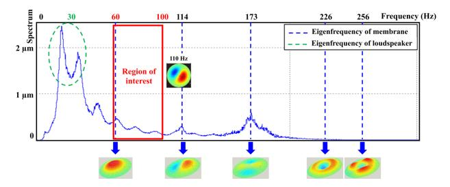
Fig. 5. Illustration of the entire membrane displacement obtained with a laser doppler vibrometer from 0 to 300 Hz associated to the frequency response spectrum. The round pneumatic driver showed the same vibration mode for the membrane only between 60 Hz and 100 Hz.
