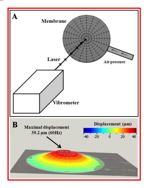
3 Fig. 1. Characterization of the membrane deformation, from 0 to 300 Hz, with a laser doppler
