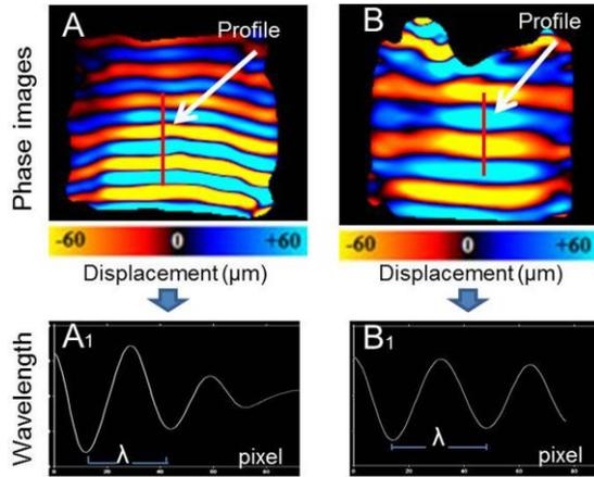
Figure 4. A-B: MRE tests were performed on both phantoms with a round driver and showed the wave's displacement inside both media. A<sub>1</sub>-B<sub>1</sub>: Behaviors of the waves traveling along the red profile.
