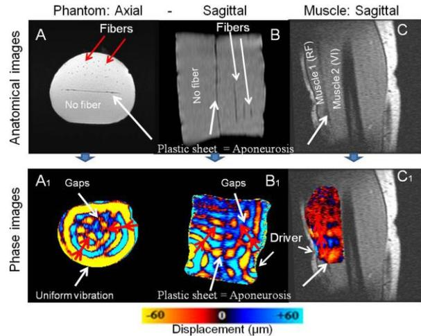
Figure 6. A-B-C: Views of the axial and sagittal anatomical images of the phantom (50%) and muscle (C). A<sub>1</sub>-B<sub>1</sub>: Result of the MRE experiments performed with the tube driver attached around the phantom. C<sub>1</sub>: MRE tests were previously performed [8] with a silicone tube driver on the selected sagittal image leading to the acquisition of in vivo phase images. Wave direction indicated by arrows along the red profile.
