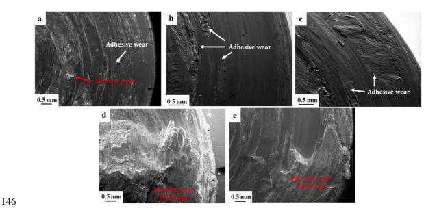
147 Figure 5 : SEM observations at mesoscopic scale for samples after galling test at 350 MPa in the case of a148 Nitronic60, b- AISI660, c- Uranus45N, d- 316L, e- 316LN
