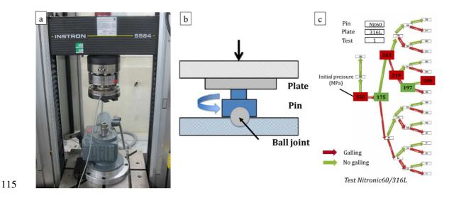
Figure 3 : a- ASTM G98 experimental galling test setup, b- schematic of the set up used for ASTM G98 galling test
