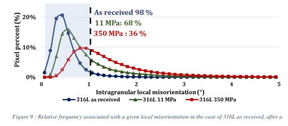
galling test at 11 MPa and after a galling test at 350 MPa
