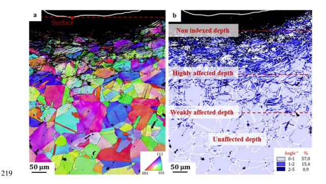
Figure 10 : a- Inverse pole figure (IPF) of 316L after galling test at 88 MPa and b- corresponding Kernel Average
