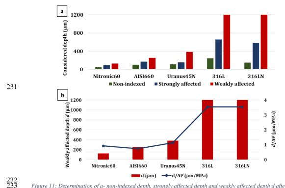
Figure 11: Determination of a- non-indexed depth, strongly affected depth and weakly affected depth d after galling
