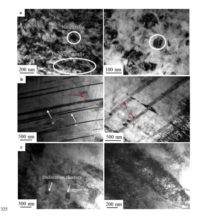
Figure 14 : TEM investigations realized in extreme surface at one of the sample's valley after a galling test realized
