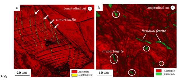
Figure 13 : Formation after a galling test realized at 350 μm of a- ε martensite inside Nitronic60 (400 μm depth) and
