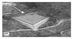
**Fig. 10.** Image of an indentation imprint of Specimen USP\_7. The image was taken with a scanning electron microscope and a tilt angle of 65°.
