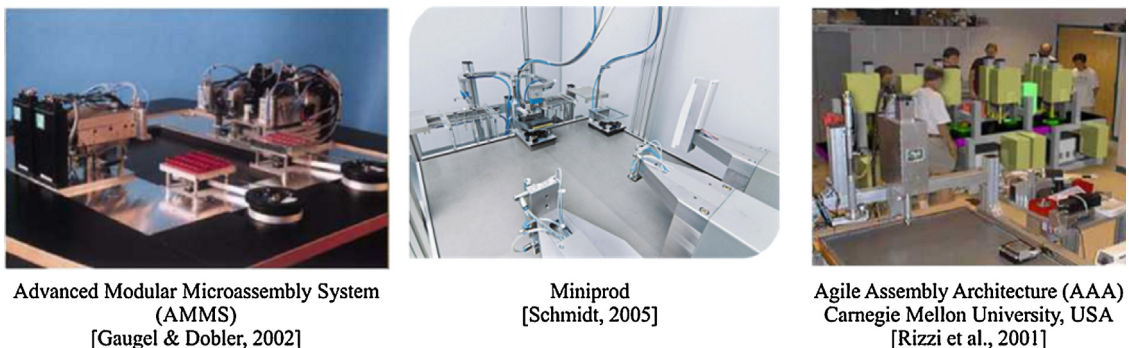
Fig. 2. Example of modular microfactory with flexible transfer line.
