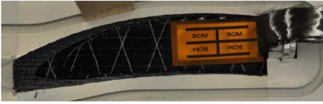
Figure 3. Picture of the piezoelectric patch embedded in the blade during the lamination process (reproduced with permission from [40]).
