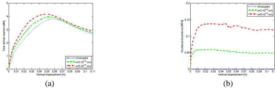
Fig. 12 Coupled soil-foundation system (a) total vertical reaction (b) excess pore pressures ( k=1 \cdot 10^{-6} m/s)
