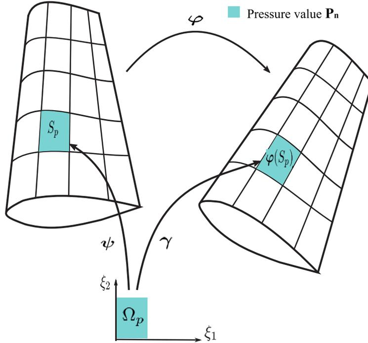
Fig. 7 Follower pressure loading: Parameterization of  $\varphi(S_p)$
