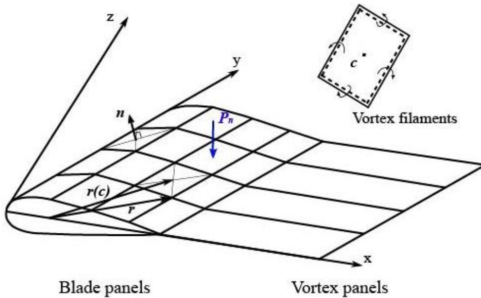
Fig. 5 Panel method mesh for wind turbine blade
