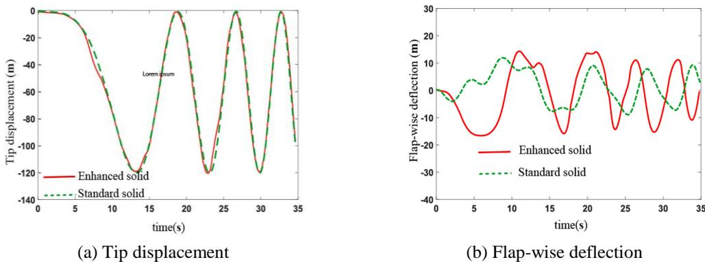
Fig. 13 Comparison between Enhanced and standard solid elements
