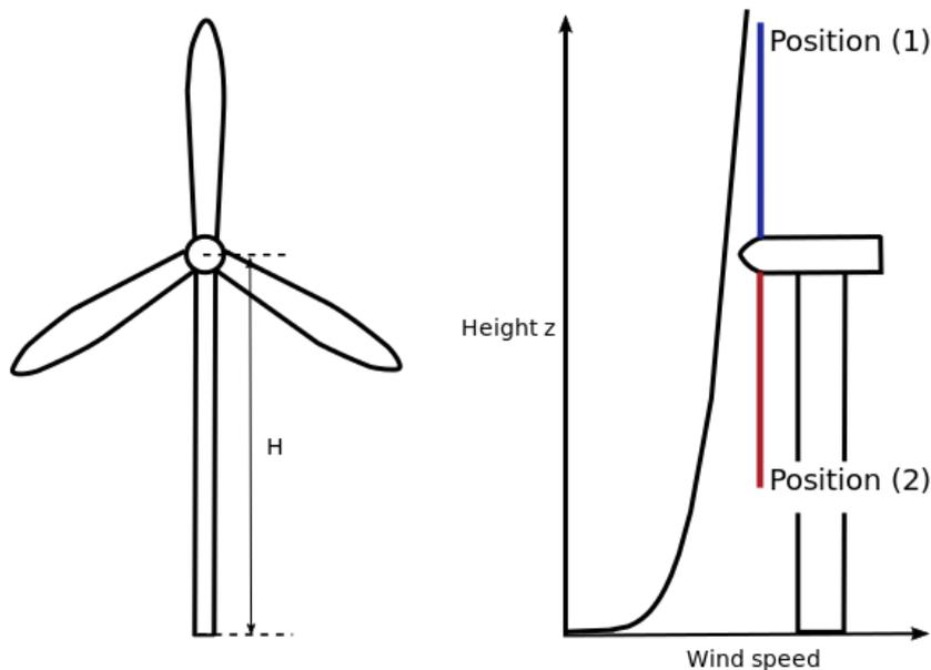
Fig. 4 Wind shear model: Variation of wind speed in height
