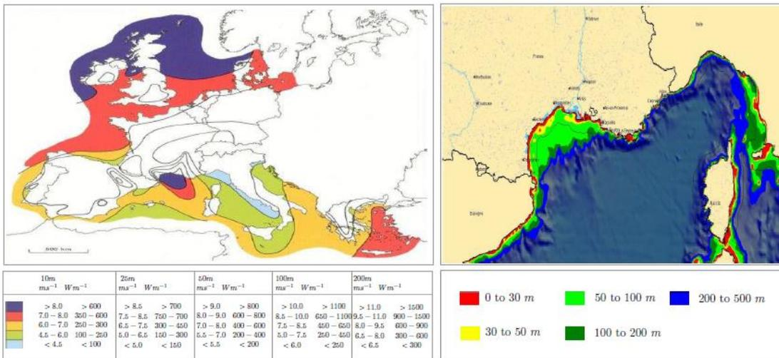
Fig. 3 Statistics on: (a) wind resources over open sea (more than 10 km offshore) for five different altitudes; (b) sea depth at different European coastal locations, showing marked difference between shallow water coast in Denmark and Germany versus deep water of Atlantic and Mediterranean coast (H. Boyé, l'éolien offshore)
