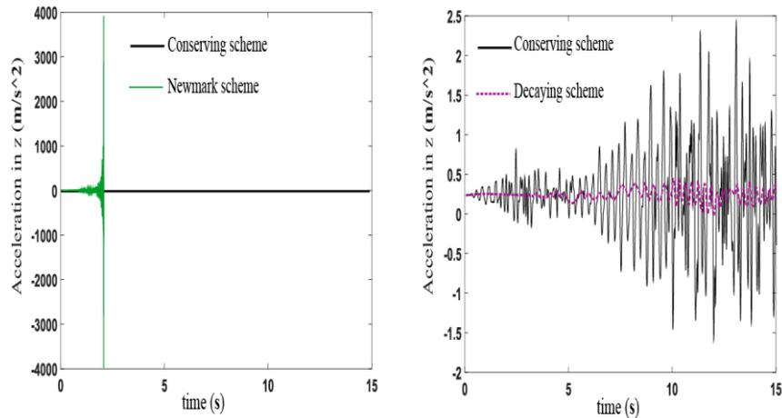
Fig. 17 Time history of acceleration in z-direction: time-stepping schemes
