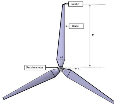
Fig. 8 Geometric model of the wind turbine
