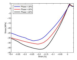
Fig. 12. Complete macroscopic response for different aggregate volume fractions.
