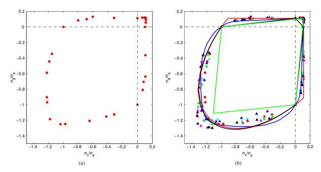
Fig. 16. Failure surfaces: (a) for realization 1; (b) for 6 realizations with the multisurface Drucker–Prager–Rankine surface (red line—Eq. (36)), coupled plasticity-damage model (black line—Eq. (37)), Saint-Venant (green line—Eq. (38)) and experimental (blue line). (For interpretation of the references to color in this figure legend, the reader is referred to the web version of this article.)
