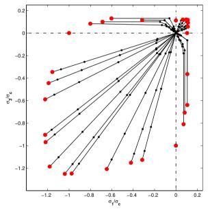
Fig. 17. Evolution of  $\sigma_1/\sigma_{ci}$  with respect to  $\sigma_3/\sigma_{ci}$  during loading until failure for realization 1 (red dots). (For interpretation of the references to color in this figure legend, the reader is referred to the web version of this article.)
