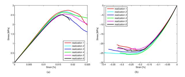
Fig. 15. Uniaxial macroscopic response for 6 realizations in plate specimen: (a) tension test; (b) compression test.
