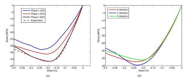
Fig. 11. Macroscopic response for uniaxial compression test: (a) different aggregate volume fractions; (b) phase I-50%.
