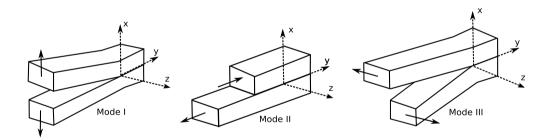
Fig. 4. Three failure modes in concrete.
