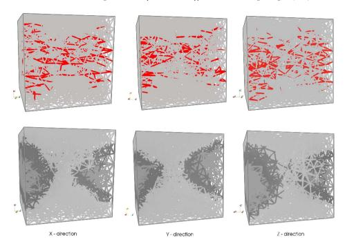
**Fig. 13.** Specimen contour at the end of uniaxial compression test for phase I-50% specimen in three loading directions. Beam elements in increasing softening are red colored (upper row), displacements in the direction perpendicular to loading direction (lower row). (For interpretation of the references to color in this figure legend, the reader is referred to the web version of this article.)
