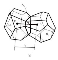
Fig. 1. (a) Structure of discrete lattice model with Voronoi cells as units of heterogeneous material and cohesive links between them; (b) two neighboring Voronoi cells.
