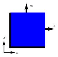
Fig. 14. Specimen for biaxial test: boundary conditions and loading.
