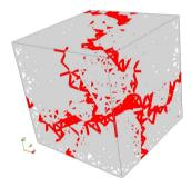
**Fig. 10.** Specimen contour at the end of hydrostatic tension test for phase I-50% specimen. Beam elements in increasing softening are red colored. (For interpretation of the references to color in this figure legend, the reader is referred to the web version of this article.)
